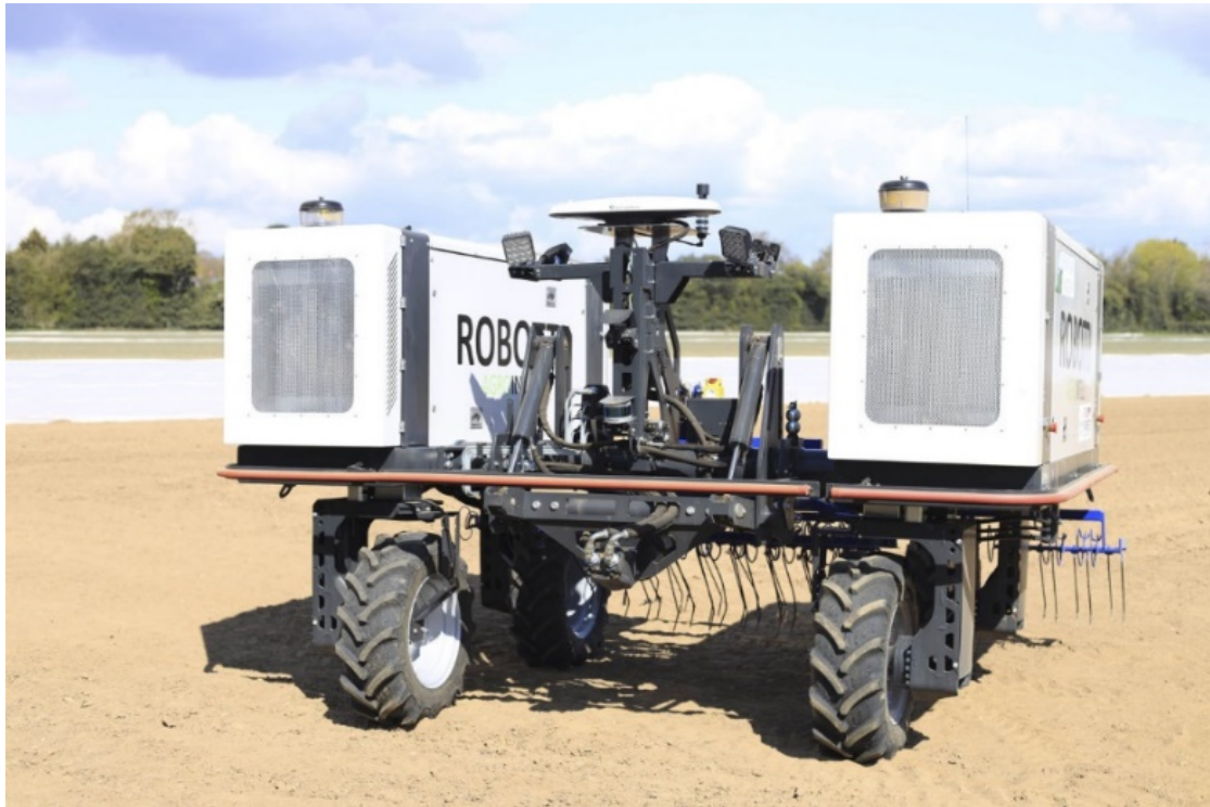
Bild 8: Autonomes Robotersystem „Robotti 150D“ von Agointelli [37] Figure 8: Autonomous robot systems “Robotti 150D“ by Agointelli [37]
